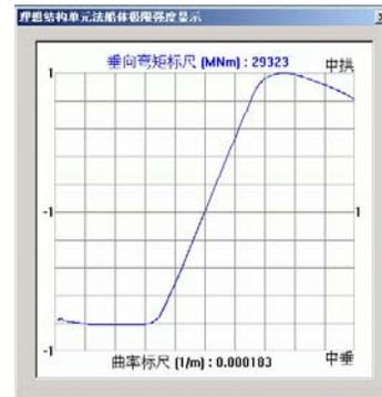
Fig.4 Bending moment and curvature relationship by ISUM
