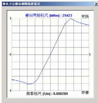
Fig.5 Bending moment and curvature relationship by SM
