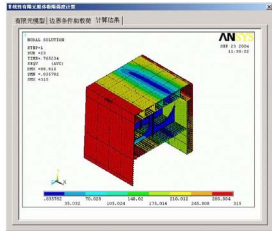
Fig.3 Equivalent stress distribution by FEM
